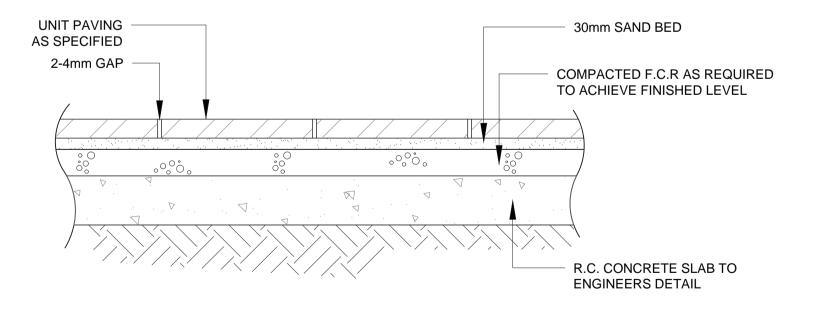
4 UNIT PAVING OVER CONCRETE SLAB
