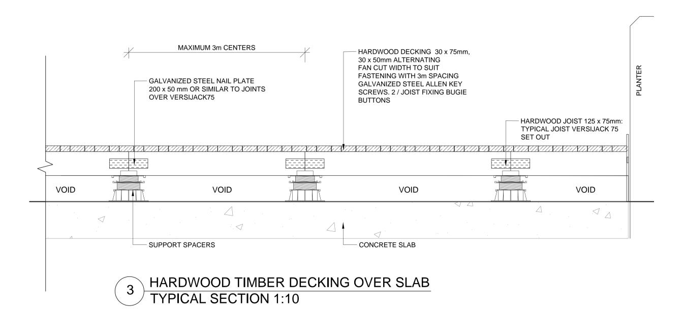
'SPOTTED GUM' HARDWOOD TIMBER BATTEN STEEL PORTAL FRAME 75X45mm +/- 10 mm FIXED TO RAILS FROM RHS 125x75x4mm ABOVE WITH GALV FIXERS MITRE JOINT FINISH: PORTER'S PAINTS COLOR: HERCULANEUM FEATURE PLANTER POTS AS SPECIFIED R.C. SLAB BY OTHERS TIMBER DECK ON VERSIJACK
