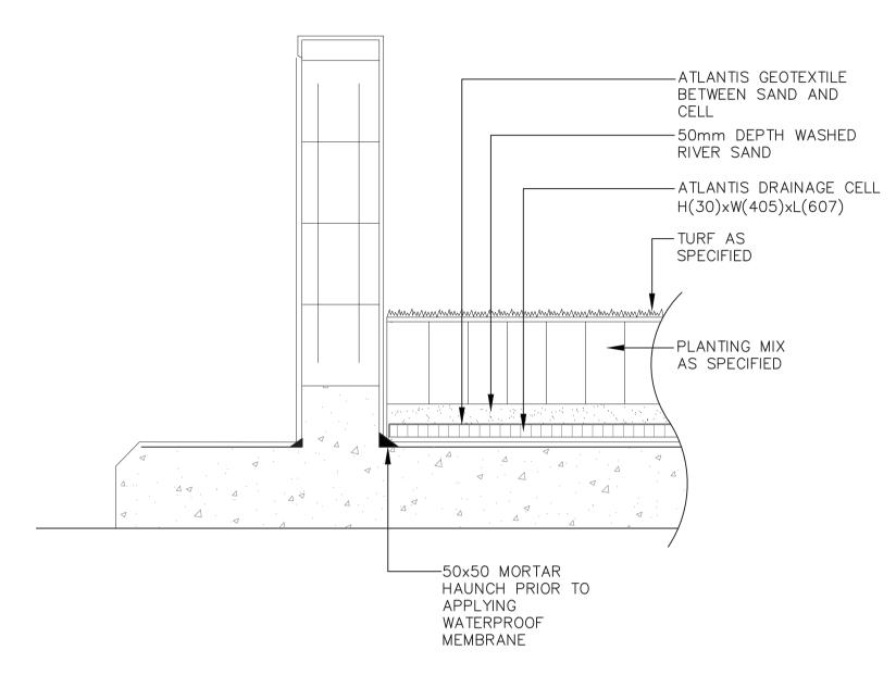
1 TURF OVER CONCRETE SLAB
